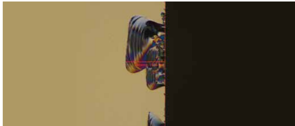
Differential interference contrast (DIC) image (2500X), the edge of chipping is clearly visible
