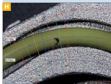
Layer thickness measurement of a curved fibre
