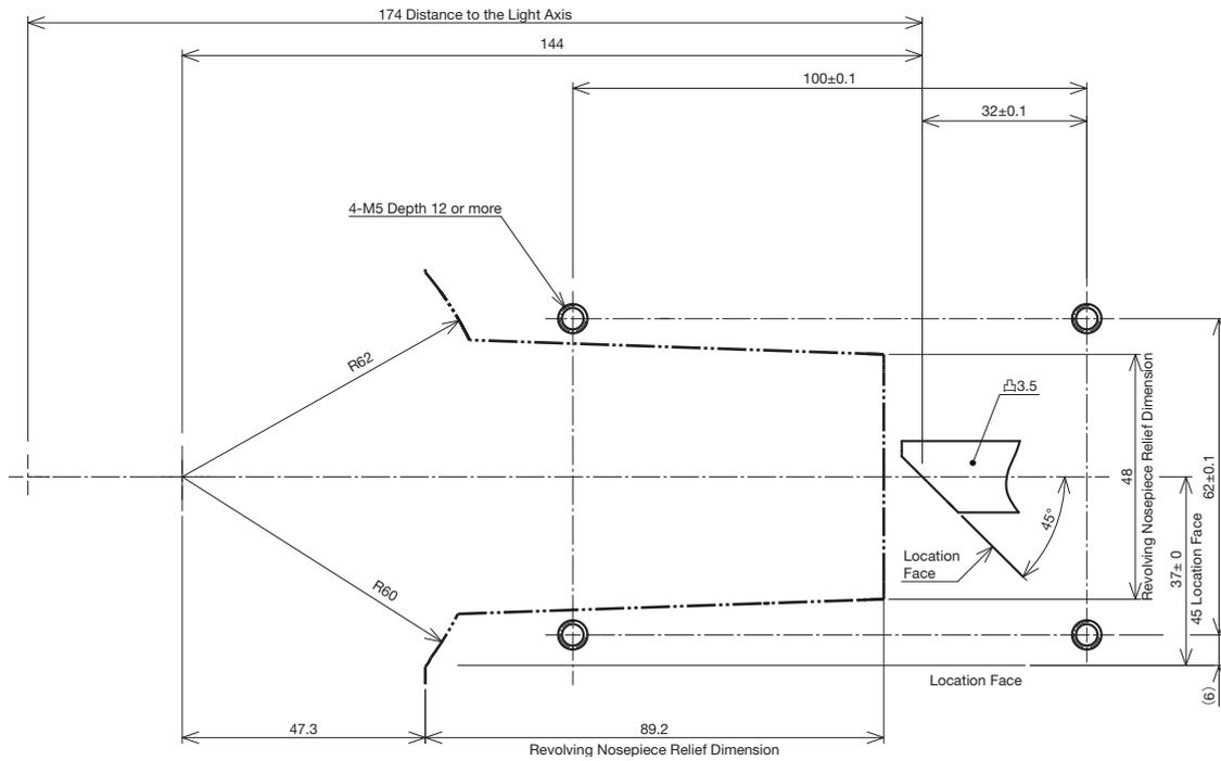
Fix illuminator using four M5 screws and projection for fastening.
