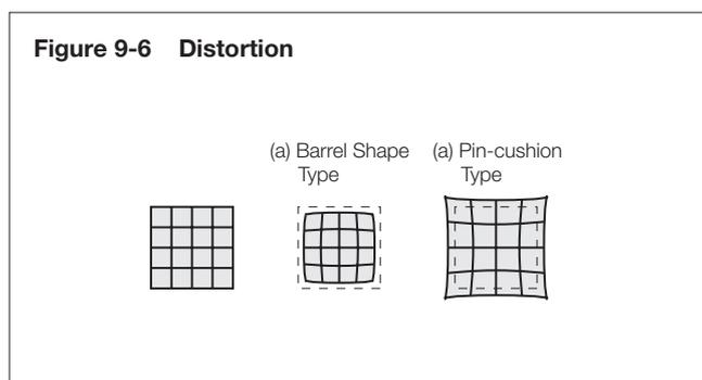
The microscope optical system contains some distortion. When distortion is present, it can bring erroneous results of shape measurements. When a microscope is used for precision measurements, pay close attention to this aberration, for example, by providing it with an aberration compensation function.
