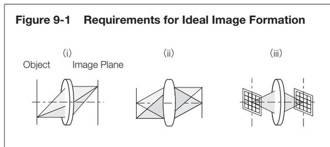
In an actual optical system, however, it is very difficult to strictly meet the requirements for ideal image formation and this causes “aberrations” that interfere with image forming performance.
