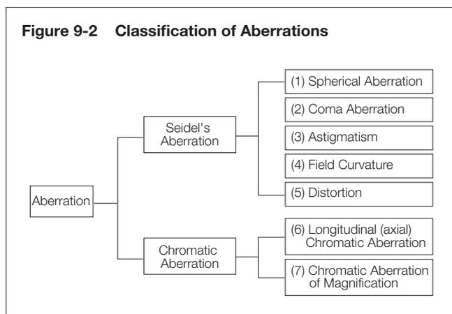
Types (1) to (3) correspond to “expansion of a point image” that goes against requirement (i) for ideal image formation in Figure 9-1. Type (4) corresponds to “curvature of image plane” that goes against requirement (ii) in Figure 9-1.
