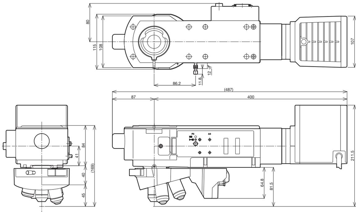
Illuminator Cable Length: 1.800 mm Weight: 5.5 kg (exclude objective)
