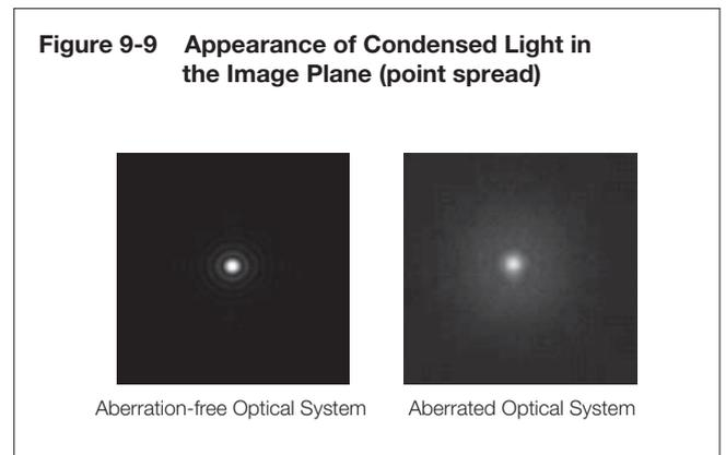
With the proportion of light concentrated in the image plane (intensity of light concentrated in the Airy disk) by an aberration-free optical system serving as 100%, the proportion of light concentrated by an aberrated optical system is known as the Strehl ratio. When graphed, the Strehl ratio reveals peaks in intensity as shown in Figure 9-10. The higher the S.R., the closer an optical system is to being aberration-free.
