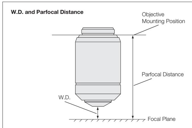
For parfocal distance of the LCPLFLN-LCD series objectives, refer to the appropriate objective page.
