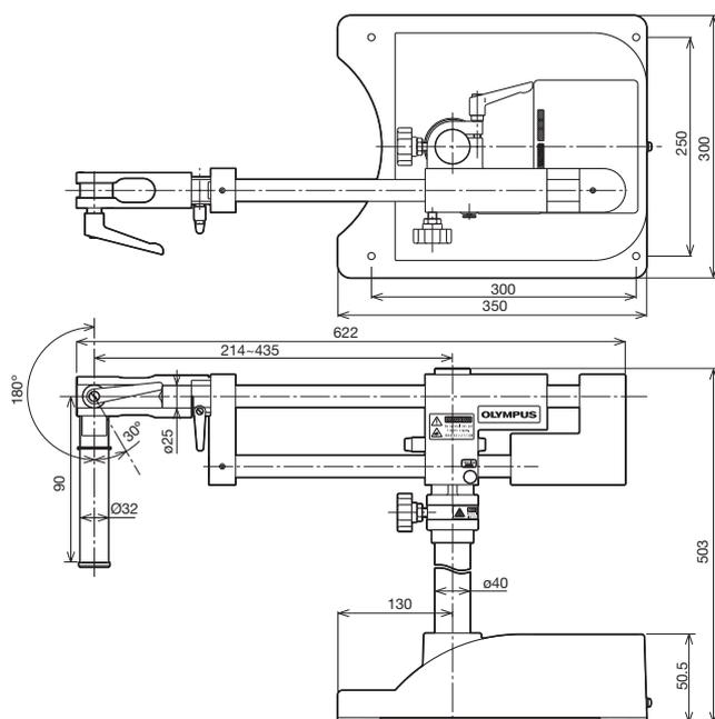
\*The rotation angle of the horizontal arm can restrict to 90 degrees with stopper.
