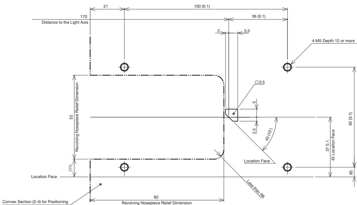
Fix illuminator using four M5 screws and projection for fastening.
