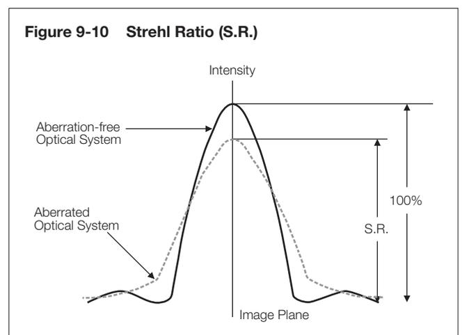
A Strehl ratio of 80% is typically called the diffraction limit, and lenses with a lower ratio lack the performance required to serve as an objective. A ratio of over 95% means that the lens' performance in general observations is comparable to that of an aplanatic lens (which is corrected for spherical aberrations and coma).
