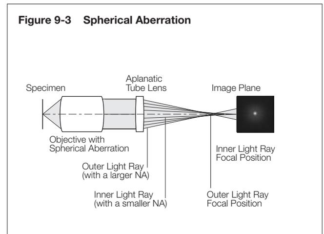
It is said that objectives with larger NA have better resolution but worsen spherical aberration. Our advanced design and manufacturing techniques have realized good optical performance even with large numerical aperture.
