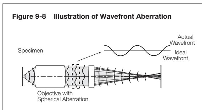
A difference (a degree of disagreement) between the ideal wavefront and the actual wavefront shown above is called “wavefront aberration.”
